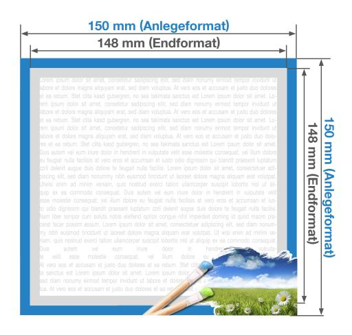
**Anlegeformat:** 150 mm x 150 mm Endformat: 148 mm x 148 mm
